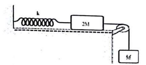
In the above figure, the system is released from rest with the spring in its equilibrium position. The pulley and the horizontal surface are frictionless. If the spring constant k = 600 N/m and M = 5.0 kg, what is the maximum extension (hairless) (in cm) of the spring?
