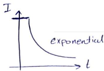
$I = I_0 e^{-t/RC}$        $I_0 = \frac{V_0}{R}$
