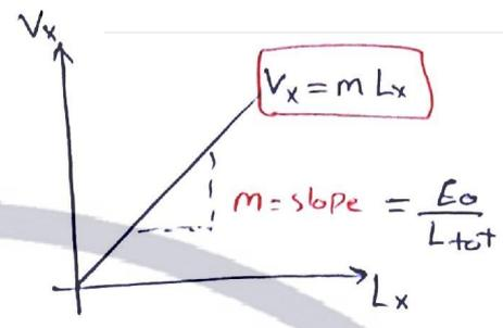
$$\begin{aligned} \rightarrow I &= \frac{V}{R} \\ &= \frac{E_0}{\frac{\rho L_{total}}{A}} \\ \rightarrow V_x &= I R_x \\ &= \frac{E_0}{\frac{\rho L_{total}}{A}} * \frac{\rho L_x}{A} \end{aligned}$$
